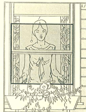
The channel guides in which vertical sliding screens operate are a permanent part of the window. They may be finished to match the trim color. Each window is numbered and corresponding number tacks are placed in sill. There is no difficulty in finding the right screen.
